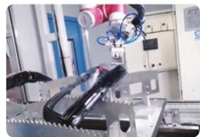
Dust removal from lighting covers
