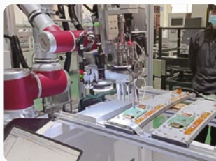
Screwing operations on lamp assembly
