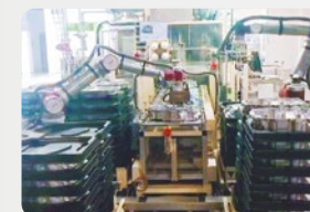
Transmission housing handling
